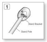
2. Insert and tighten three large screws (5x15, For connecting Stand Pole & Stand Bracket) into the three holes on the Stand Bracket as shown in the illustration.
